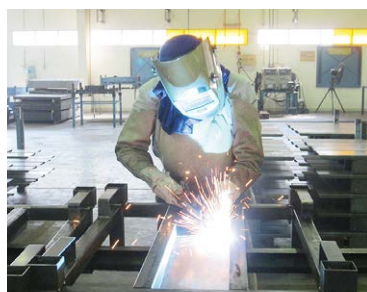
Manufacturing of large pallets for machinery transportation
