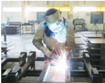
Manufacturing of large pallets for machinery transportation
