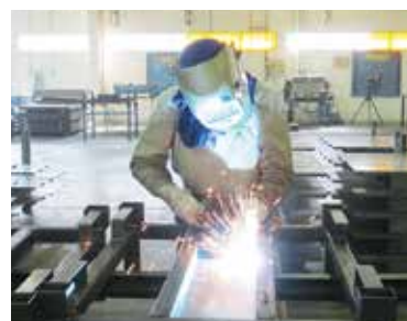
Manufacturing of large pallets for machinery transportation
